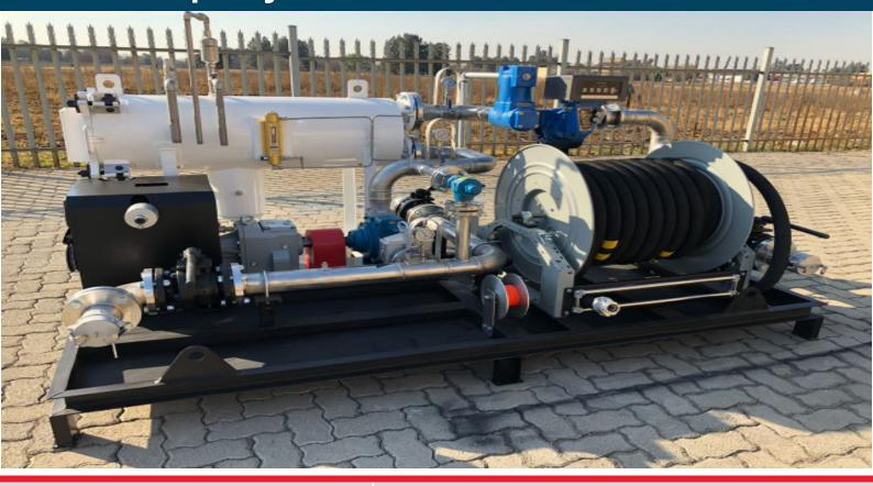
Capable of down-loading, uploading and circulating Diesel fuel at 500 l/min without the need of disconnection or reconnection of site hoses.
